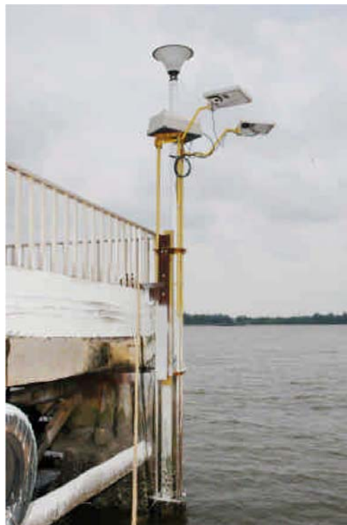
Figure 1. Internet-enabled real-time reporting sea-level gauge installation at Verem Naval jetty (Mandovi estuary, Goa).
