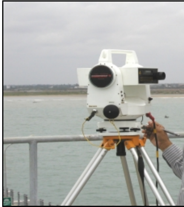
Fig :1 Figure shows “Laser Trak” an optical instrument mounted on a Tripod stand, used for measuring angles and distances from shore based locations.
