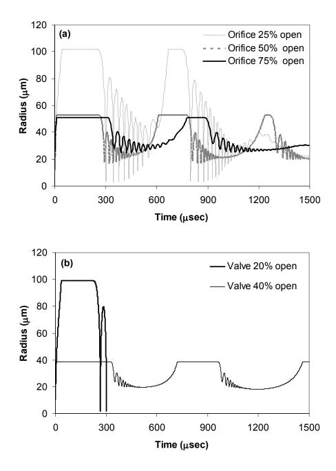
**Fig. 5** - Cavity dynamics of 10µm cavity (a) orifice configurations (b) valve configurations
