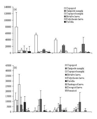
**Fig. 6** - The influence of cavitating conditions created by (a) differential pump valve opening and (b) created by flowing through a cavitating element (orifice plates) on the survival of zooplankton.
