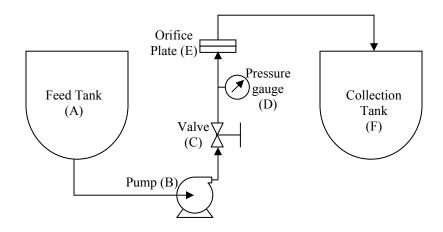
**Fig. 1** - Schematic of the experimental set up (A - Feed tank; B- centrifugal pump; C-Flow regulating valve; D- Pressure guage; E- Cavitation element (Orifice); F- Collection tank)
