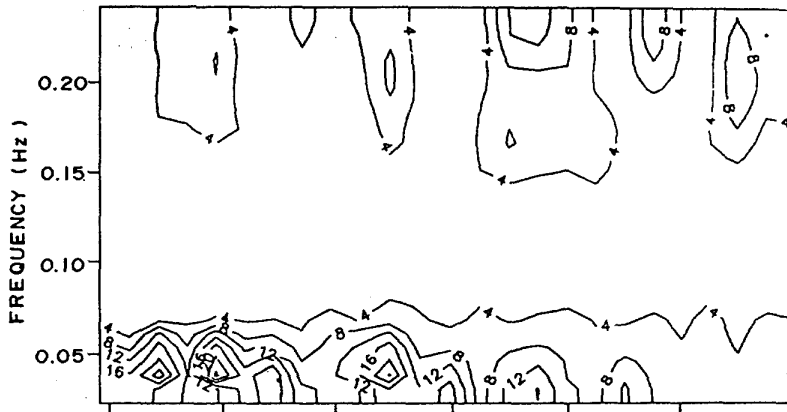
Fig. 3a Standard deviation of a maximum of 15 redundant estimates (gauge triads) of wave direction (degrees) at Duck during 1-6 February 1994.
