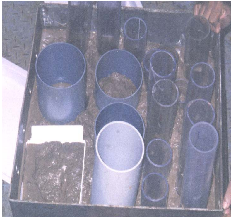
Fig.2. Sub-sampling of macrofauna from the box corer.
