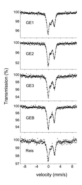
Figure-1 Mössbauer Spectra of the glass samples from Lonar Crater region. See Table-1 for interpretations of the Sample Codes.
