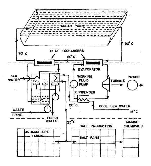
Fig. 1 The solar pond (top) absorbs solar energy. The hot water from the lower layers of the pond is circulated through the power plant (middle right) and the desalination plant (middle left).
