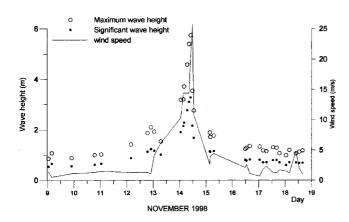
**Figure 2.** Variation of maximum wave height  $(H_{\text{max}})$ , significant wave height  $(H_s)$  and recorded wind speed with time.
