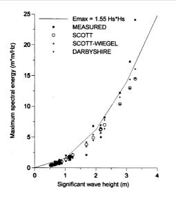
Figure 8. Variation of maximum spectral density measured and estimated based on Darbyshire, Scott and Scott-Wiegel with significant wave height.
