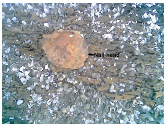
Figure 4. Figure showing the nail head and deposition of bivalves on the wooden stock.
