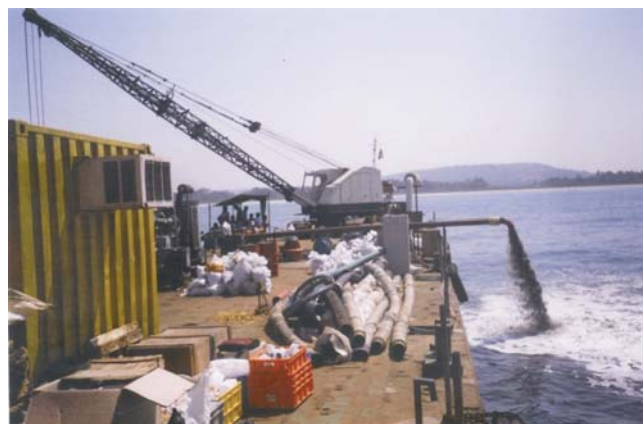
Figure 3. Placer mining experiment (PLAMEX-I) off Kalbadevi Bay, Ratnagiri. Note the suction (station S) and discharge points (station D) are on opposite sides of the Pontoon (left and right respectively), and the photo is taken from the reference point (station R, Photo by ABV).
