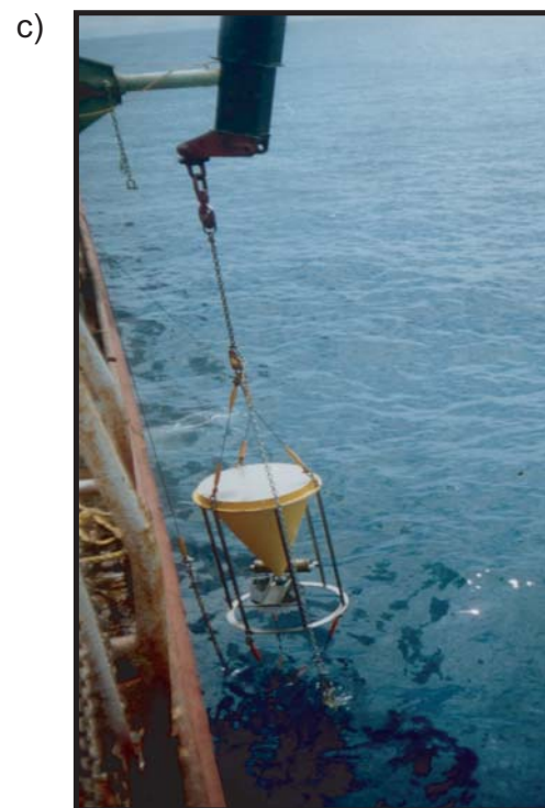
Fig. 4.7. a) Photograph showing three sphere radio float with glass floatation spheres at the surface before retrieval. b) Photograph showing the retrieval of sediment trap array. c) Photograph showing the retrieval of sediment trap.
