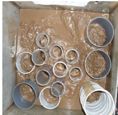
c. Sediment sample in box corer
