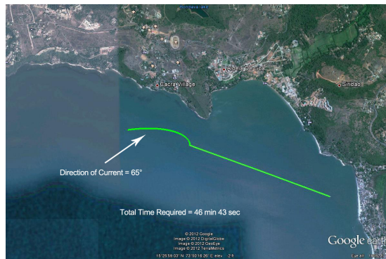
Fig. 10 Simulation of Maya following a straight path in the presence of tidal current
