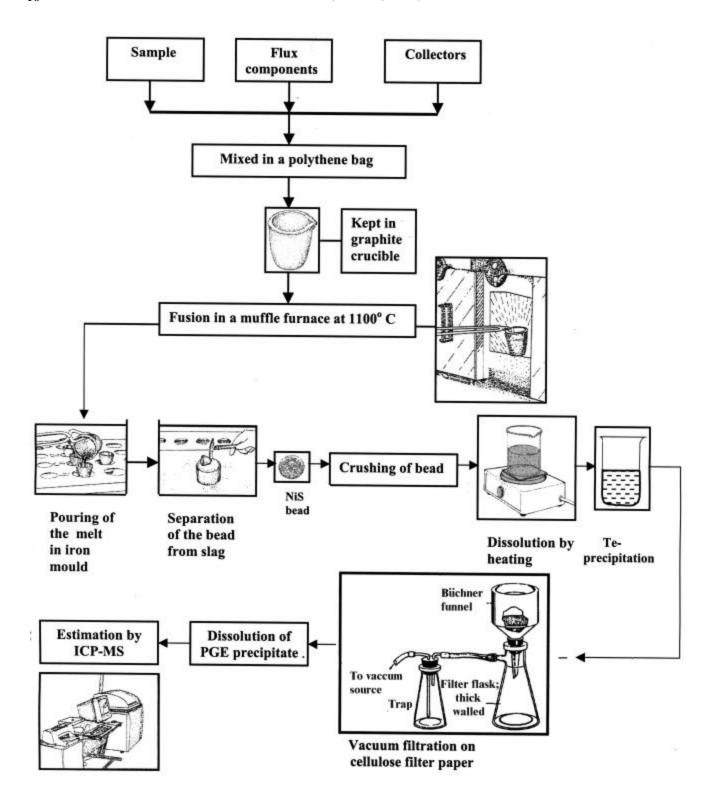
Fig. 1—Schematic representation of various steps involving separation, preconcentration and ICP-MS determination of PGE and Au in international manganese nodule reference samples.
