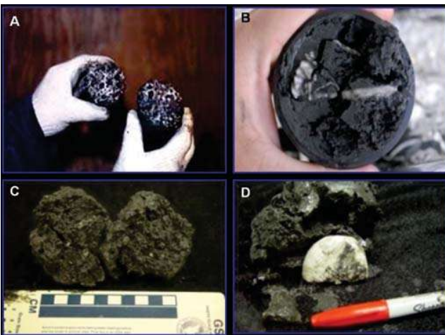
Figure-4. Mode of occurrence of Gas hydrate from a sediment sample retrieved from KG basin East coast of India in which hydrate occurs in various modes: (A) Nodules; (B) Laminae/Veins; (C) Grains; (D) Massive. (Source: NGHP-01 expedition, India).
