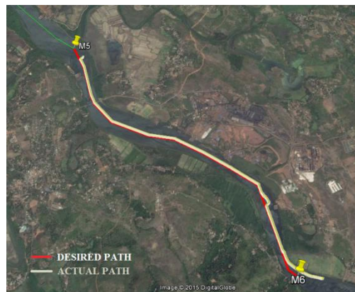
Fig 5. Actual and desired path of MAYA
