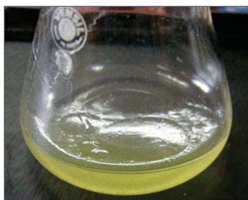
Figure: 2 Formation of Emulsion in Saponin test
