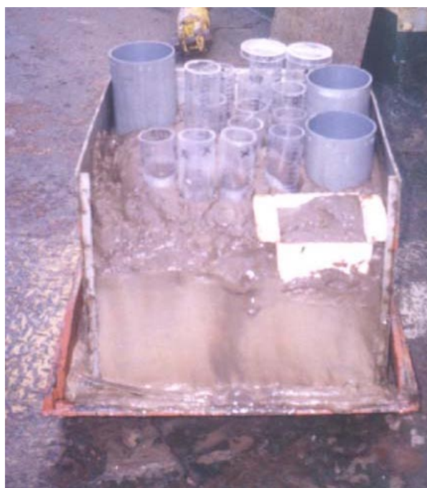
Figure 1. Photograph showing sub-cores of different diameters (2.5 and 5.7 cm) inserted in the sample box of box corer on-board A. A. Sidorenko (AAS-46).
