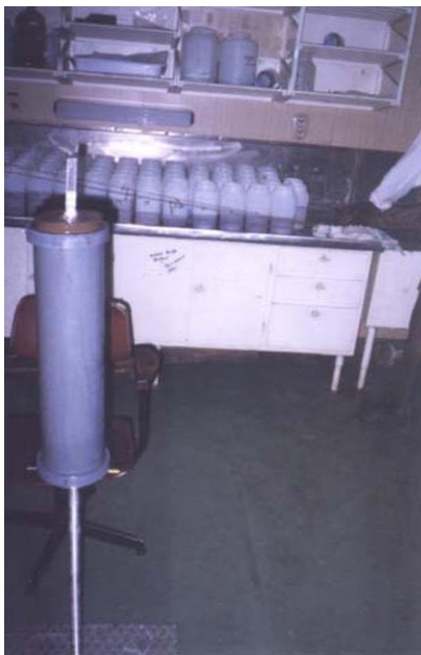
Figure 5. Photograph of the sediment sub-sampler used on-board R/V A.A. Sidorenko during AAS-46 cruise (2002). Sediment displayed on the top of the sub-core (5.7 cm dia.) is 2 cm thick. The steel scale in the background is to verify the thickness of the sediment to be sectioned.
