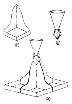
The splitter consists of a funnel and four pans (Fig. A), designed in such a way that the funnel is welded to the edges of the four angular ridges that are formed, within which the adjacent sides of the pans fit in clegantly, thus avoiding spilling while the splitter is in operation.
