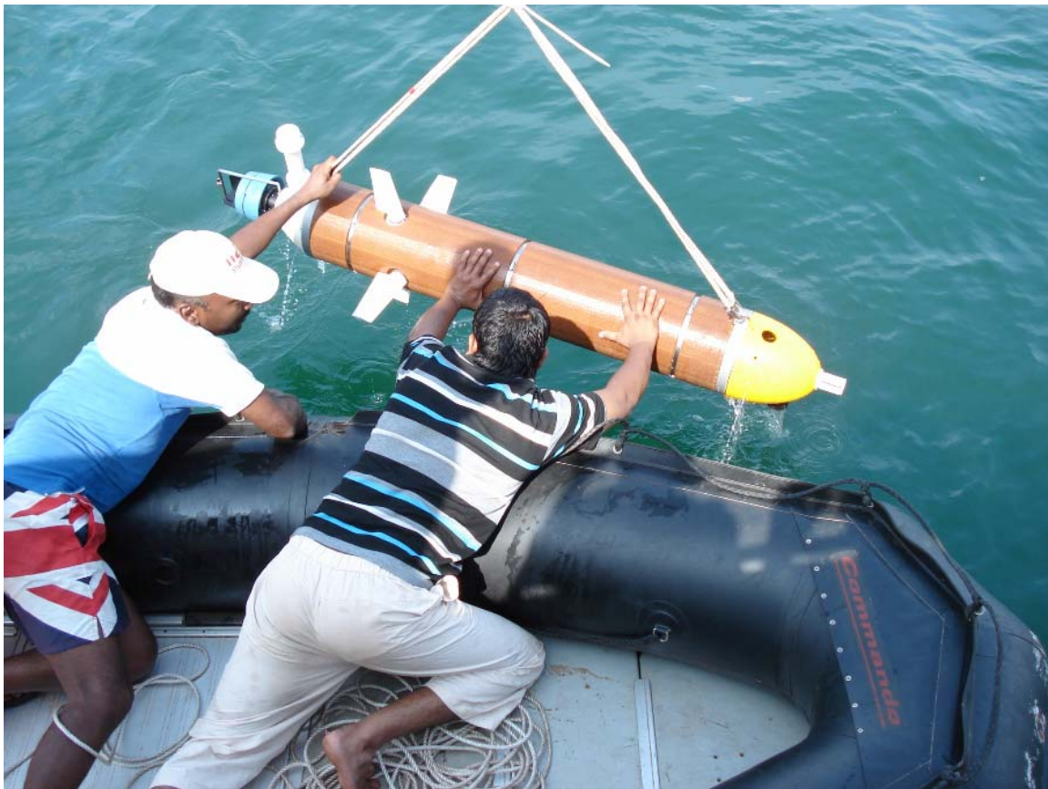
Fig 6: Retrieval method of the Maya AUV using an inflatable craft.
