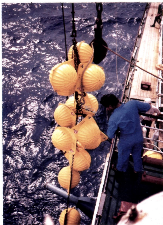
Fig. 46 (a) Deep - sea mooring being recovered on Sagar Kanya.
