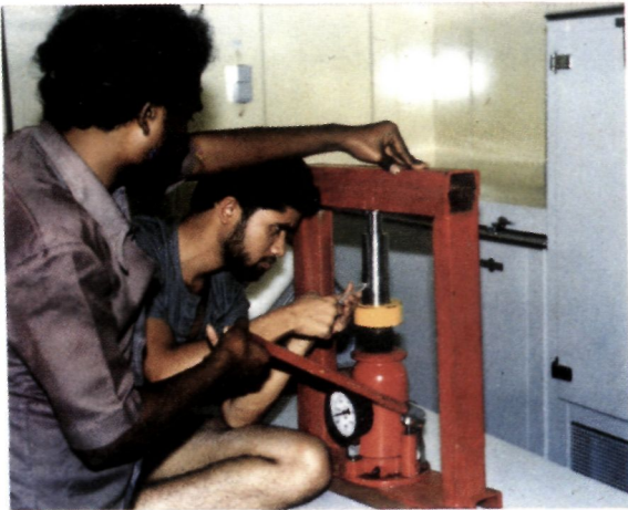
Fig. 44 Modified squeezer for pore water extraction from sediments.
