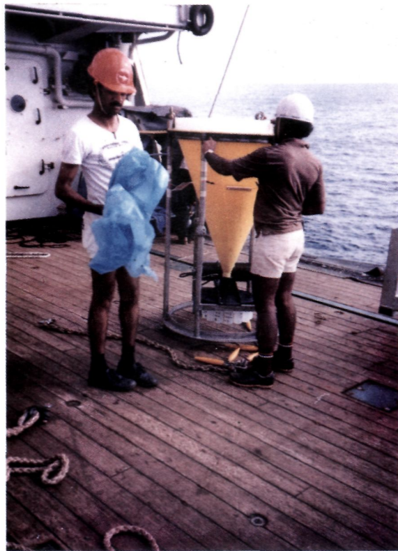
Fig. 46 (b) Sediment trap on deck of Sagar Kanya.
