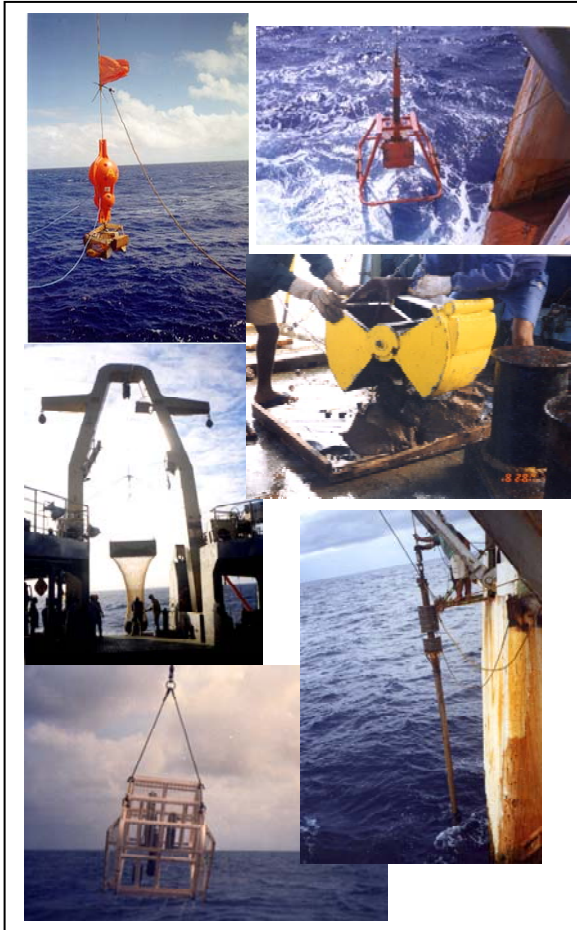
Fig. 4 Various sampling equipments used, clockwise: A : Free fall grab or a boomerang grab; B: Space corer; C: A gravity corer; D : Deep towed camera system; E : Dredge used for bulk sampling of nodules
