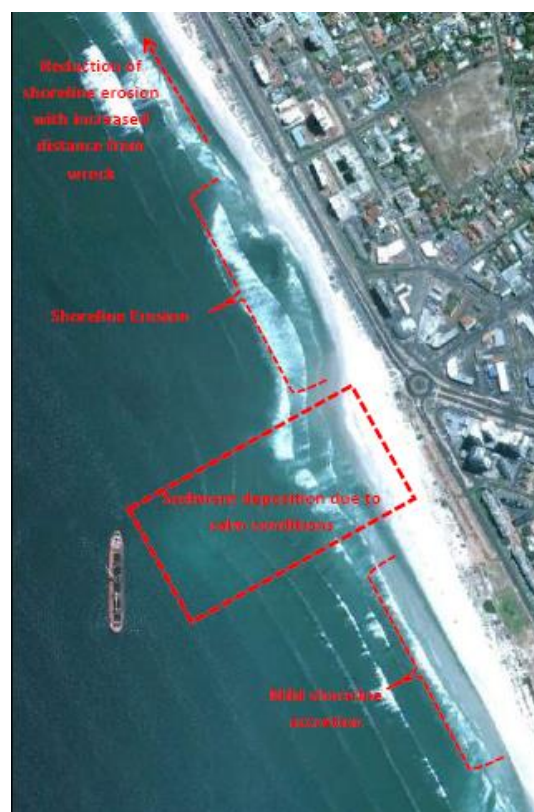
Fig 5—A detailed presentation of post grounding effects of Seli One in Blouberg, Cape Town, South Africa; sediment deposition, erosion and accretion are clearly demarcated after Seifart 6 .
