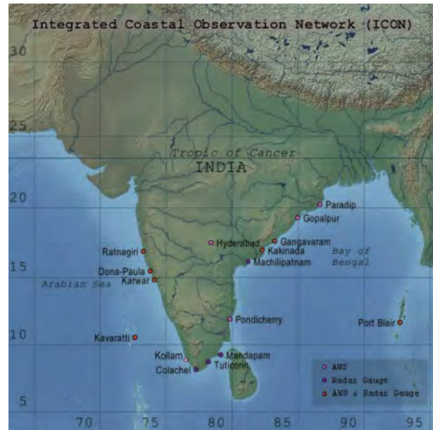
Figure 1. Radar based sea-level gauges and autonomous weather stations installed along the Indian coasts and islands.
