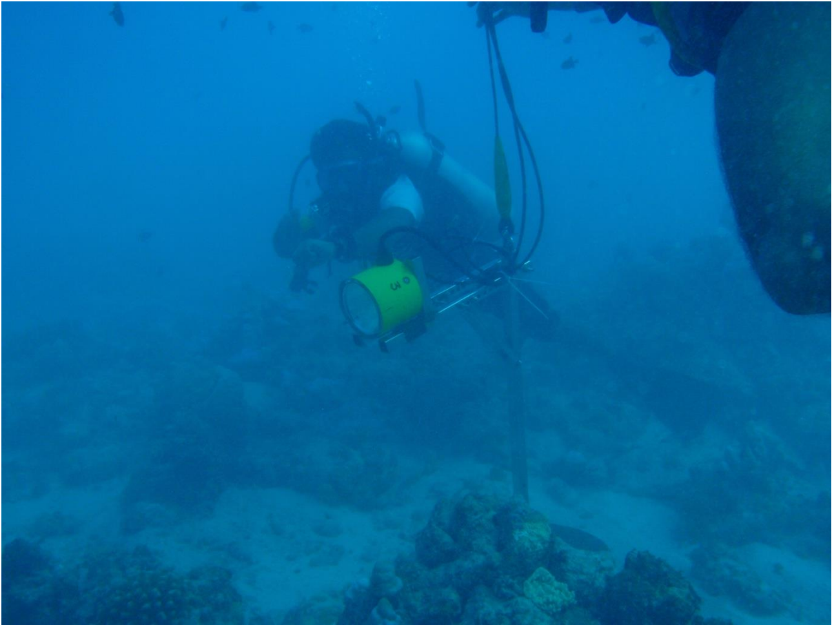
Figure 5: The Image Acquisition Unit (IAU) deployed at the seabed in the vicinity of a coral cluster.
