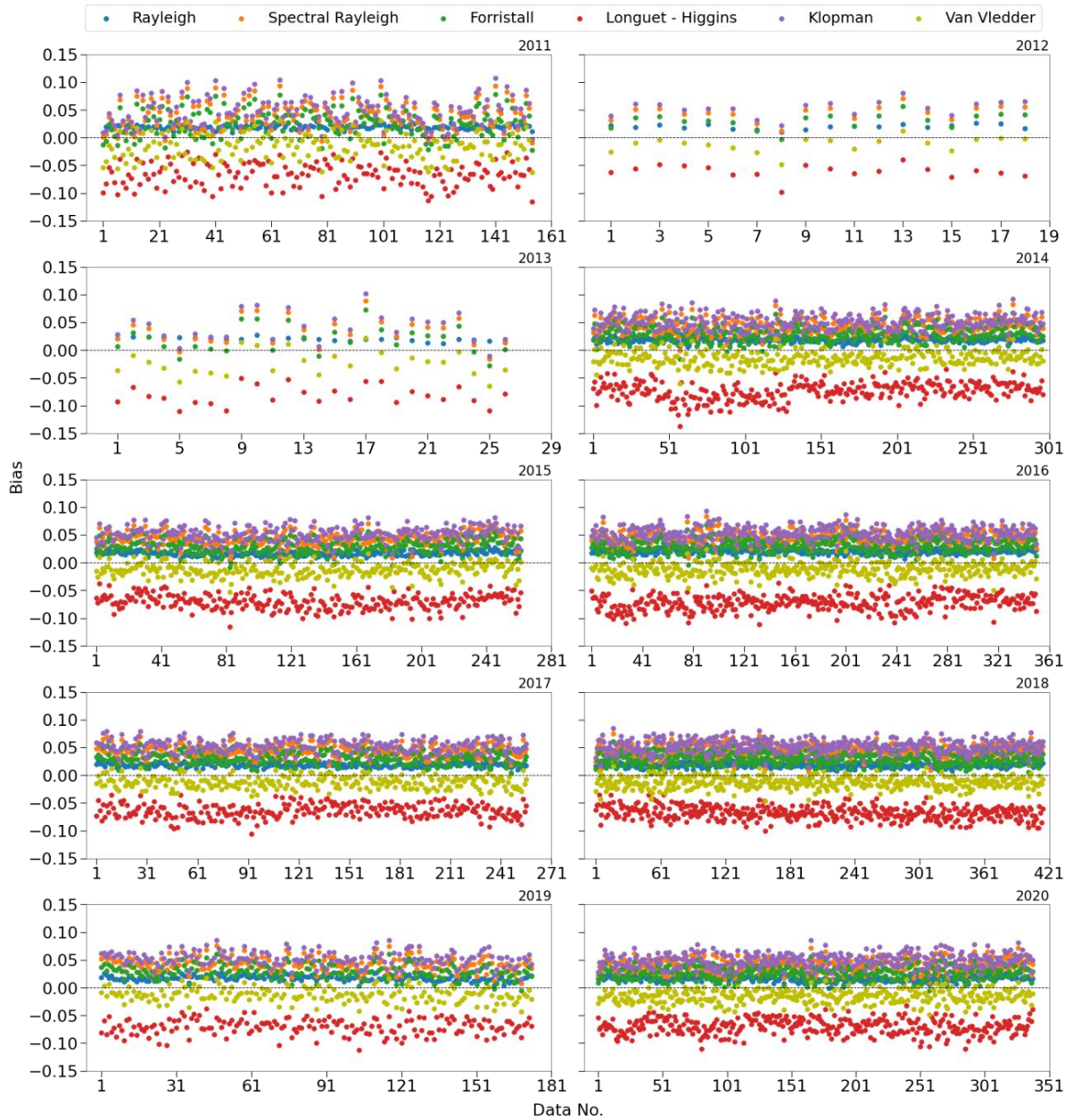
Fig. 10. Bias between observed wave height data and the distribution models calculated for each 30-minute record with significant wave height ( H_{1/3} ) greater than or equal to 3 m. Each plot represents various years from 2011 to 2020.
